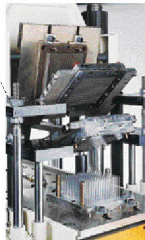
4RT special mold open system - press can automatically separate multi-plate molds and clean mold easily.
